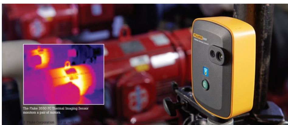
Fluke 3550 with an image capture of two motors
