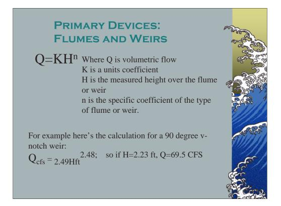
Here's the equation for flumes and weirs. Note how critical the measurement of H, liquid level, is. There are many tables of coefficients and examples of how to calculate flow. Flow transmitters all have equations built into them.
