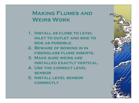
For a flume or weir to be accurate, it must be installed properly. Most error problems with open channel flow measurements are traceable to the accuracy of the flume or weir, not the level measurement or the flow transmitter.
