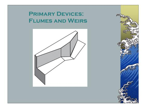
Flumes have a constriction in the flow, and a "hydraulic jump" that causes the head height to be linear and repeatable. There are dozens of kinds of flumes. In modern times, the most common are the Parshall and the Palmer-Bowlus flumes.
