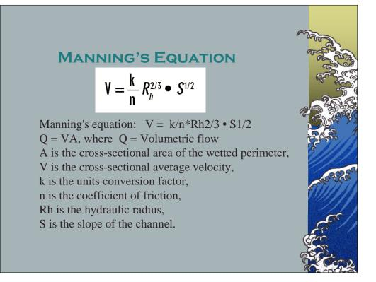
In 1889, Irish engineer Robert Manning produced an equation for calculating flow in open conduits from the level in the channel.
