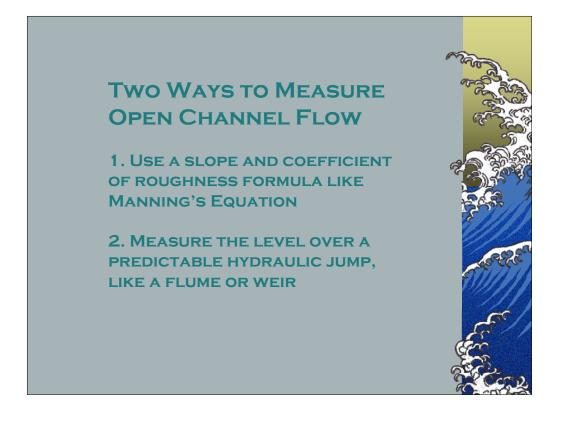
There are two basic ways to measure flow in an open channel or conduit.
