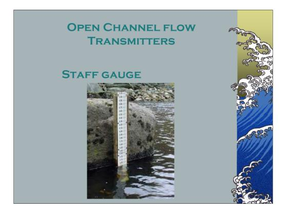
Just like its ancient predecessor, the Nilometer, the staff gauge is a ruler stuck in the flow with its end point at the arbitrary zero flow point. It is read by the calibrated MK I Eyeball.
