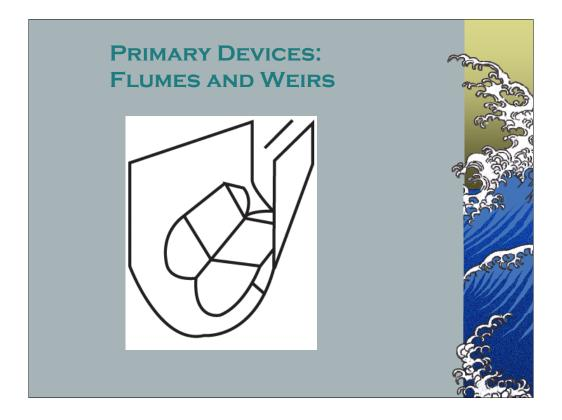
Palmer-Bowlus flumes were originally developed for measurement in sewers and other open conduits with relatively low flow. There is no constriction, as with a Parshall flume, but there is a complex hydraulic jump that forms the point where the height is directly proportional to flow rate, the "H" in our equation.
