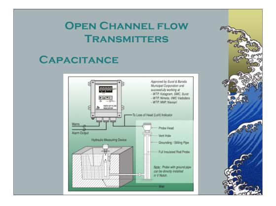
You can still find capacitance or RF Admittance Flow Transmitters for open channel flow, like this one. The capacitance or admittance changes with the level on the sensor, and the level signal is then converted to flow. These sensors have lots of issues, especially with grease or foam in wastewater or irrigation, but they work very well in small flumes and weirs.
