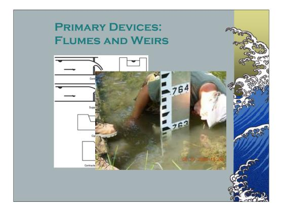
Note that I said flow transmitter not flow meter. That's because the primary device is itself the flow meter. All the transmitter does is to automate the staff gauge. As with the Nilometer, a primary device can measure flow using the calibrated Mark 1 eyeball. What the various types of flow transmitters do is to make it unnecessary for somebody to stand there and eyeball the primary device.
