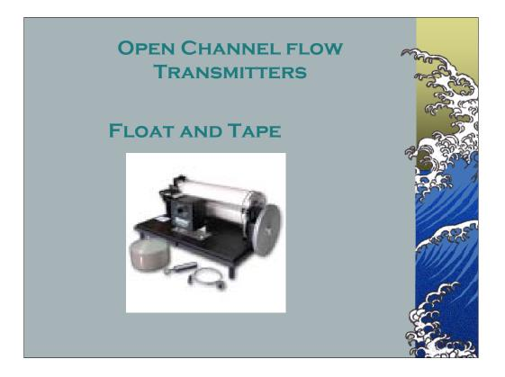
Originally a purely mechanical measurement, with a windup chart recorder, float and tape flowmeters are still in use all over the world, mostly for stream gauging for organizations like USGS. The movement of the float drives a cam operated pen across the chart. Simple, effective, accurate, and doesn't require power. The operator winds the chart motor every week or so, when he comes to change the chart.
