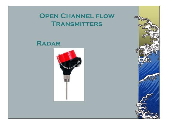
Both guided wave and downlooking radar transmitters have been used for open channel flow where wind or other interference makes it impossible to use ultrasonic flow sensors.
