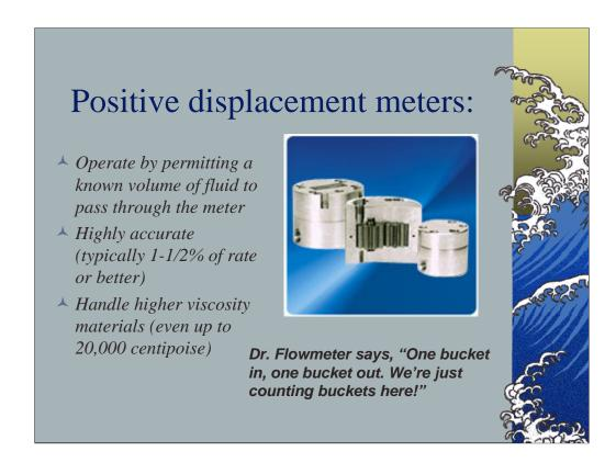
Positive displacement meters are used for both liquids and gases...and are nearly always highly accurate. They come in a variety of types, such as oval gear, reciprocating piston, nutating disc, rotary piston, and they all work by emulating a bucket. One bucket in, one bucket out.
