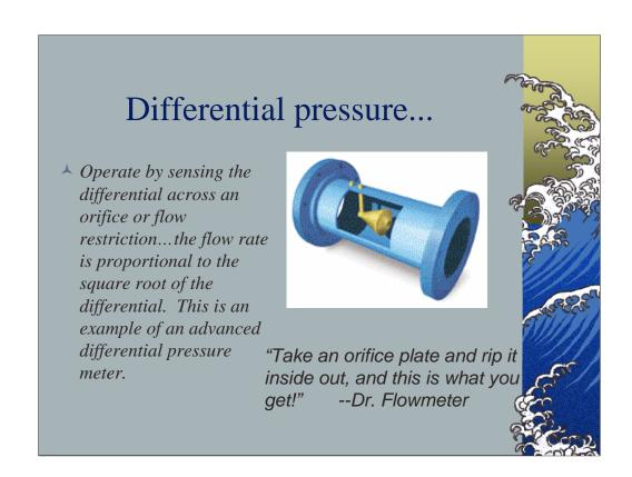
Differential pressure based flow measurement is still the widest used technique throughout the process industries. Why? It is simple, inexpensive, and is accomplished with the use of pressure transmitters, which the plant usually has for other measurements (pressure and level) anyway.
