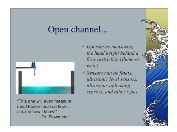
In an open channel application, the "flow meter" is the flow restriction itself: the flume or weir. The instrument is only the level sensor used to automate the meter reading. You can use a yardstick and be quite accurate.
