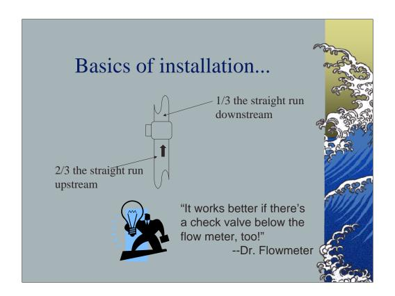
Putting a flow sensor into a vertical line with flow going up usually makes it work better even in disturbed flow profiles too, because you are using gravity to help develop the profile. A vertical riser installation usually helps combat entrained air or gases in a liquid stream, too.
