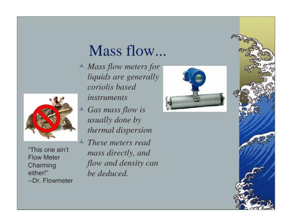
If I were told that I had to pick two types of flow meters to use, forever, and only two; and that I would be judged based solely on the accuracy of the measurement, I'd surely pick a coriolis mass flow meter as one of the two. A spool piece style magmeter would probably be the other one.
