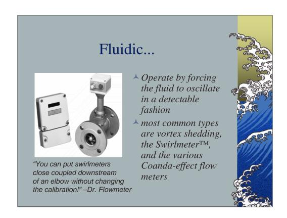
Vortex shedding meters and other fluidic types have no moving parts and use the fluid itself the way a turbine uses its rotor. A traditional vortex shedding meter uses a bluff body (often called a shedder bar) to produce the repeatable oscillation. A Swirlmeter uses a stationary "rotor-like" device to twist the flow and a restriction to contain and make the oscillation repeat. The Coanda-effect meter uses hydraulic feedback to force the fluid to oscillate in proportion to velocity.
