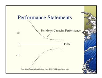
Performance expressed as a percent of calibrated span is similar to full scale and meter capacity statements where the absolute error is a percentage of the calibrated span
