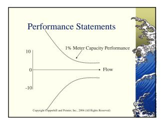
Performance expressed as a percent of calibrated span is similar to full scale and meter capacity statements where the absolute error is a percentage of the calibrated span
